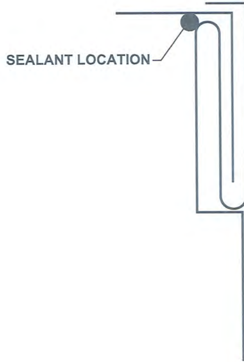
Pittsburgh Lock Seam for Duct
