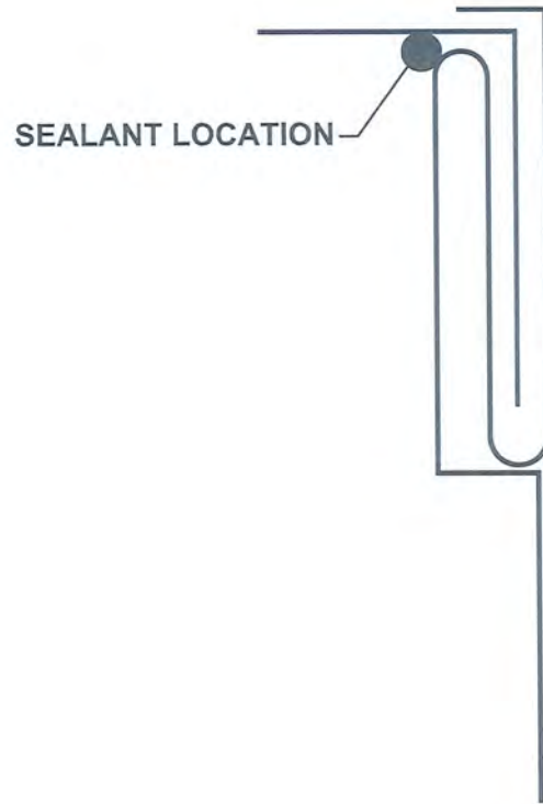
Pittsburgh Lock Seam for Duct
