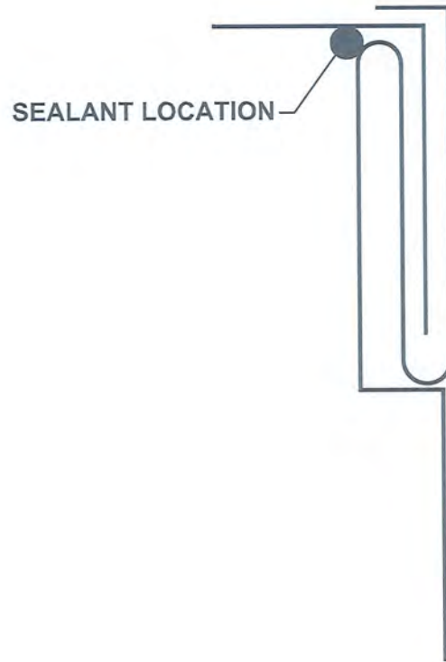
Pittsburgh Lock Seam for Duct
