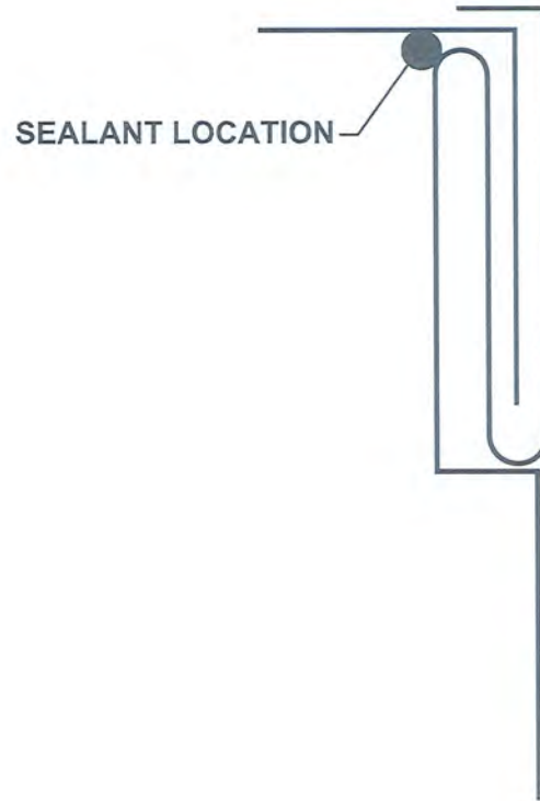
Pittsburgh Lock Seam for Duct
