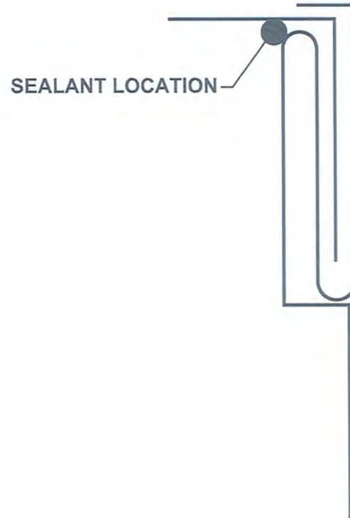
Pittsburg Lock Seam for Duct
