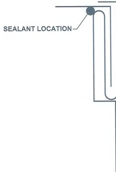
Pittsburgh Lock Seam for Duct
